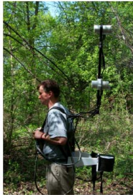
Fig 6. GEM GSM-19W Magnetometer system, configured with 2 sensors for gradient measurements Ref [48]
