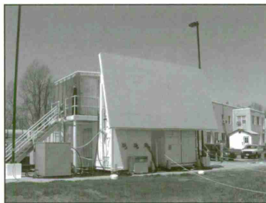
The Advanced Multifunction RF Concept (AMRFC) test bed is a proof-of-principle demonstration system capable of simultaneously transmitting and receiving multiple beams from common transmit and receive array antennas for radar, electronic warfare, and communications.
