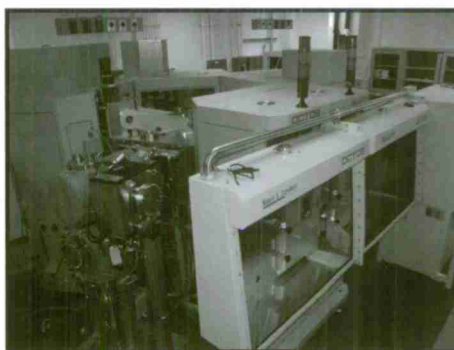
The Advanced Optical Materials Fabrication Laboratory, a state-of-the-art high vacuum cluster system, consists of a series of interconnected chambers allowing vacuum deposition of complex, multilayer films to be deposited and patterned without breaking vacuum during processing.
