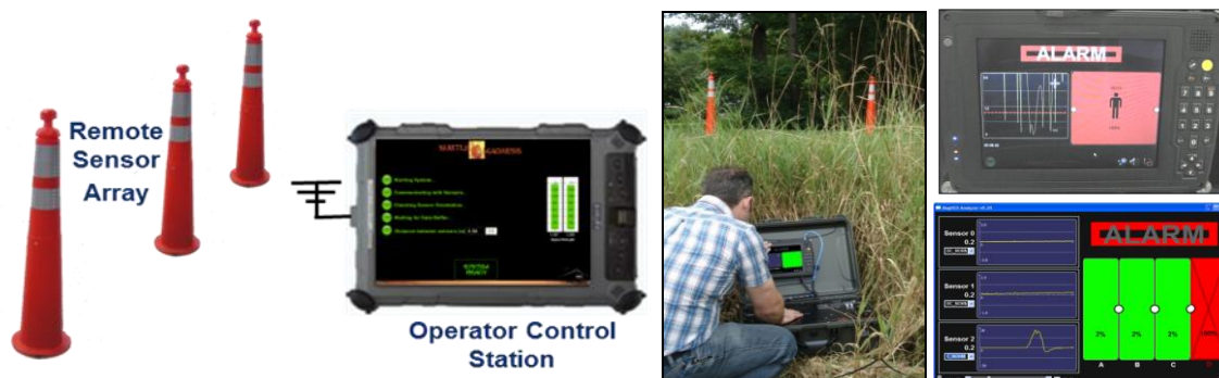
Figure 2. Left-to-Right: The two primary system components: 1) remote sensor array concealed in traffic cones and 2) operator control station (OCS). Photo of OCS with power transmitter (foreground) remoted from sensors (background). Photo (top) and screen capture (bottom) of SubtleMadness display in single gate screening mode (two sensors) and trip wire mode (multiple sensor nodes). In the trip wire mode, the system displays the zone of the alarm as well signaling audible tone for the operator at the OCS location.
