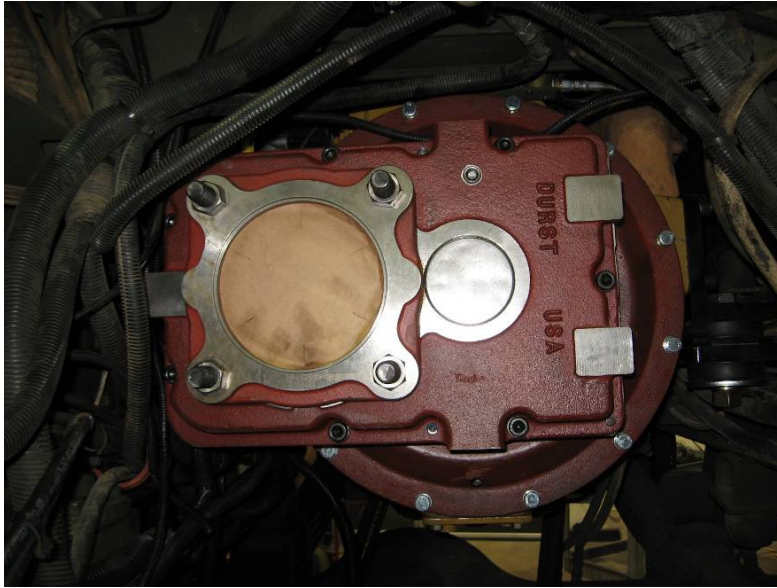
Figure 3.4.1-2. Durst Gearbox Mounted on Engine
