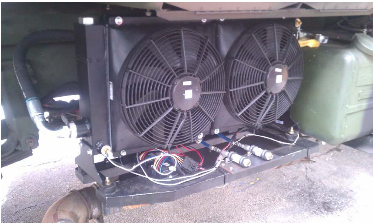
Figure 3.4.2-3. Hydraulic Oil Cooler
