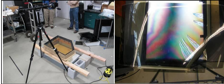
Figure 3. The two standard methods utilized to establish the camera sensor plane parallel to the sample face plane. The use of a tripod, left-hand image, or a mono stand is best. Space and sample size can preclude using the first two methods, leaving a safety ladder as the alternative, as shown on the right. Note the bow in the analyzer film.
