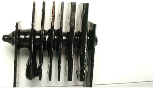
FIG. 2—The end-of-test coupon assembly of corrosion test D 1384 for nano graphite (Acheson Aquadag E) in Zerex G-05/water (left) and Zerex 618/water (right).
