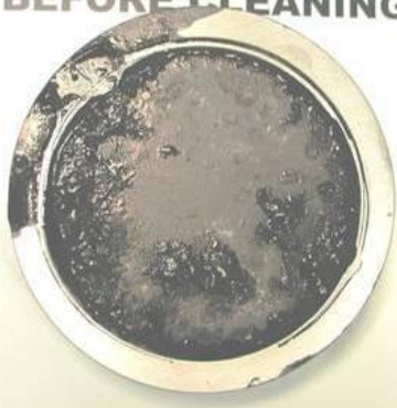
FIG. 3—The end-of-test specimen of corrosion test D 4340 for nano graphite (Acheson Aquadag E) in Zerex G-05/water (left) and Zerex 618/water (right).
