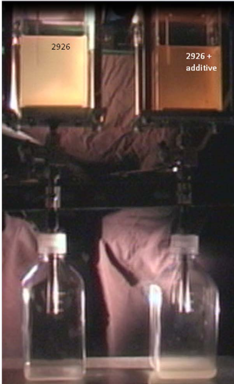
Figure 25. Photograph of test vessels upon completion of static condition and gravity flow testing of neat Jet A (Left side) and Jet A with 2,000 mg/L LT additive (right side)
