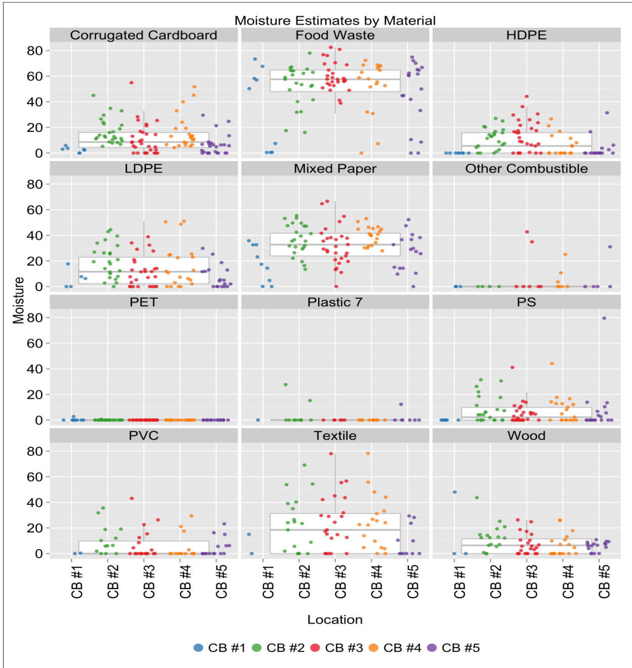
Figure D.1. Moisture Content Readings by Waste Component Category
