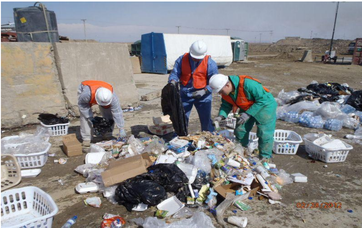
Figure C.2. Example of Manually Sorting a Sample by Waste Type (Component Categories)
