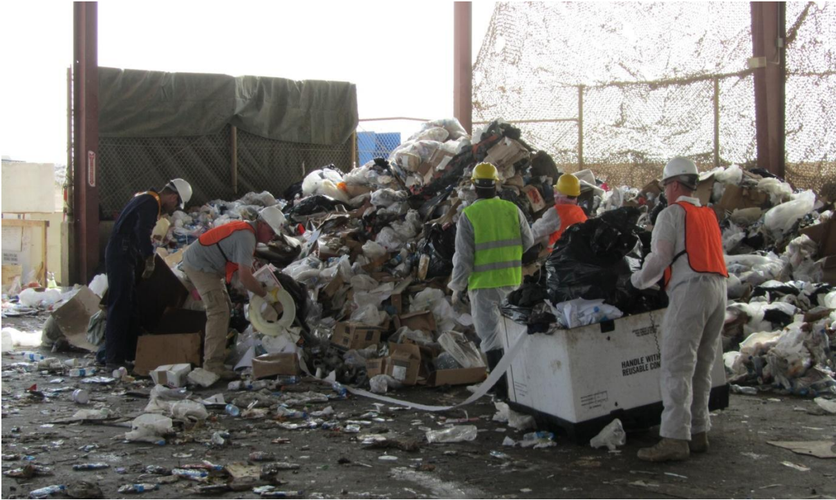
Figure C.1. Example of Collection of a >200lb Mixed Waste Sample
