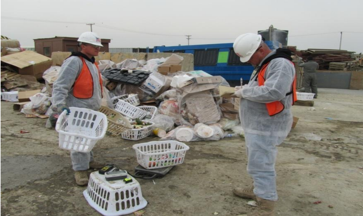
Figure C.3. Example of Field Measurements of Waste Component Characteristics (Note the portable scale and the black and yellow moisture meter on top of the basket in foreground)
