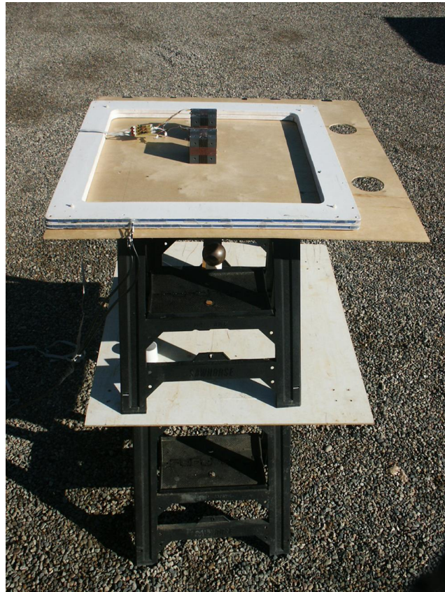
Figure 39: Picture of experimental setup. The near cube is located at the center of the transmitter loop. The far cube offset by 20 cm. The Z coils (vertical axis) were used on each cube.
