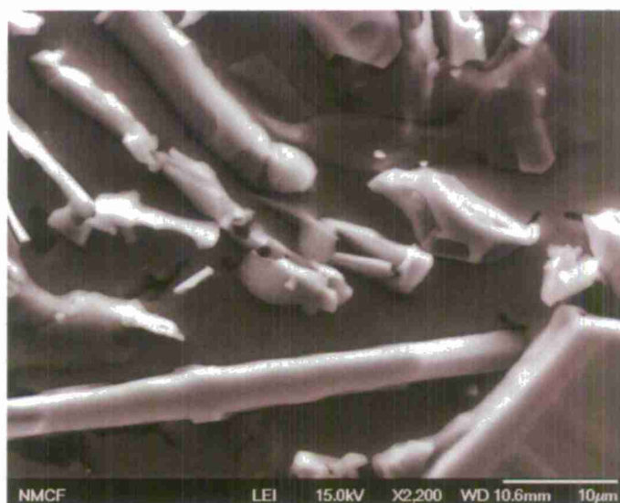
Figure 15. Region 1 (braze) UNS A96061 T6 + UNS A94047 (BA1Si-4) wedge reheat treated to T6. Shown is a post immersion micrograph of an initially mechanically polished and electropolished sample that was SEM imaged and then mechanically polished 5 μm. This sample was immersed for 8 hour immersion test in acidified salt water (BS 11846 Method B solution), cleaned and imaged.
