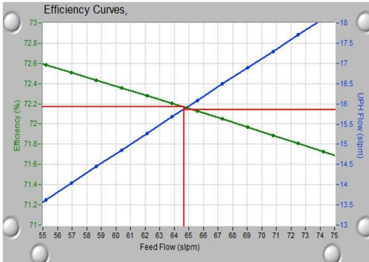
Figure 1: P&E expected UPH flow from the reformat composition, flow and operating pressure 15.9 slpm hydrogen.
