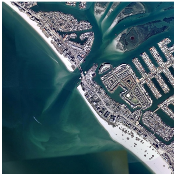
Figure 3. The attachment point of Johns Pass ebb-tidal delta. Note the wide beach at and south of the attachment and narrow beach north. The aerial photo is taken in 2007.
