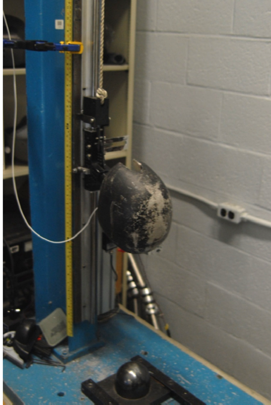
Figure 14. Monorail drop test with DOT-Size C headform and hemispherical anvil
