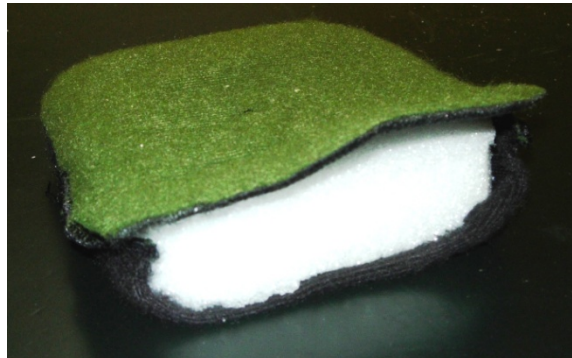
Figure 27. ROHACELL® foam replaced in fabric pad covering
