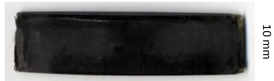
Top view of [90,0]_s healable composite
