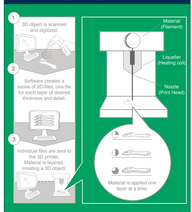
\* Fused Filament Fabrication (FFF) is only one example of the many available 3D printing processes. As building materials such as metals, food, and tissue cells become more sophisticated, so do the manufacturing processes and machines.
