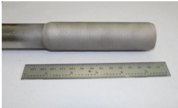
Figure 10. Picture of Stellite 25 tube with nickel cold-sprayed at one end (not machined).
