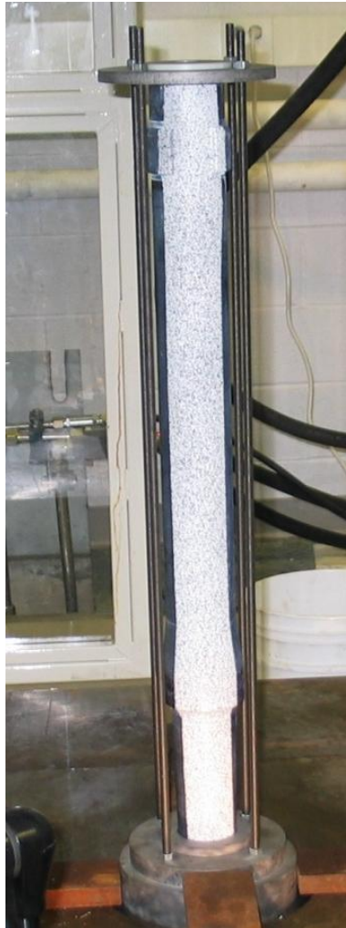
Figure 6. Truncated gun tube in GLEEM testing fixture at full scale.
