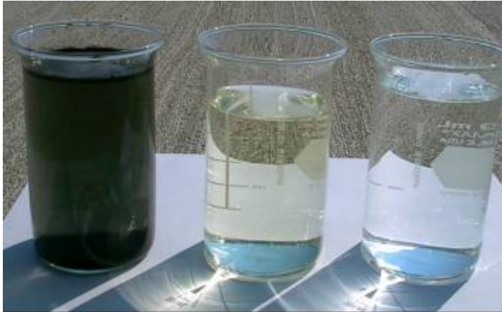
Exhaust condensate Particle Filtered Water Carbon/Resin Purified Water Figure 3: As-received and purified exhaust condensate
