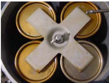
Figure 1. Coalescers/Separators Mounted in a DOD housing
