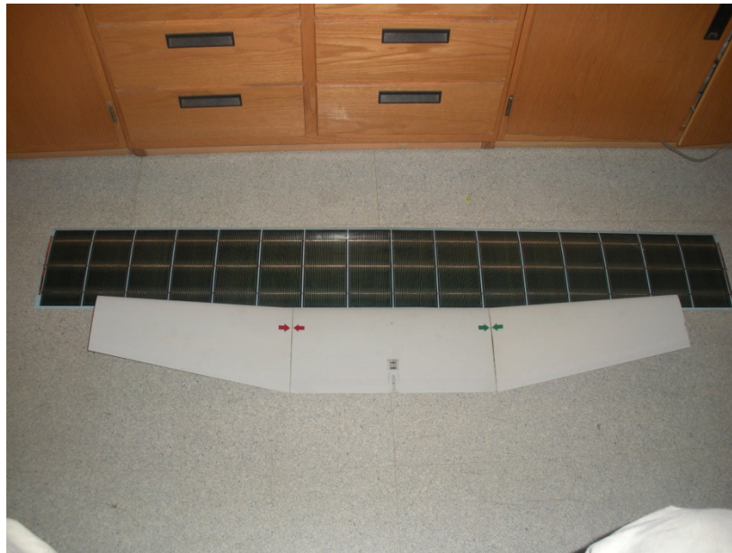
Figure 41. Completed array above the original Raven wing.
