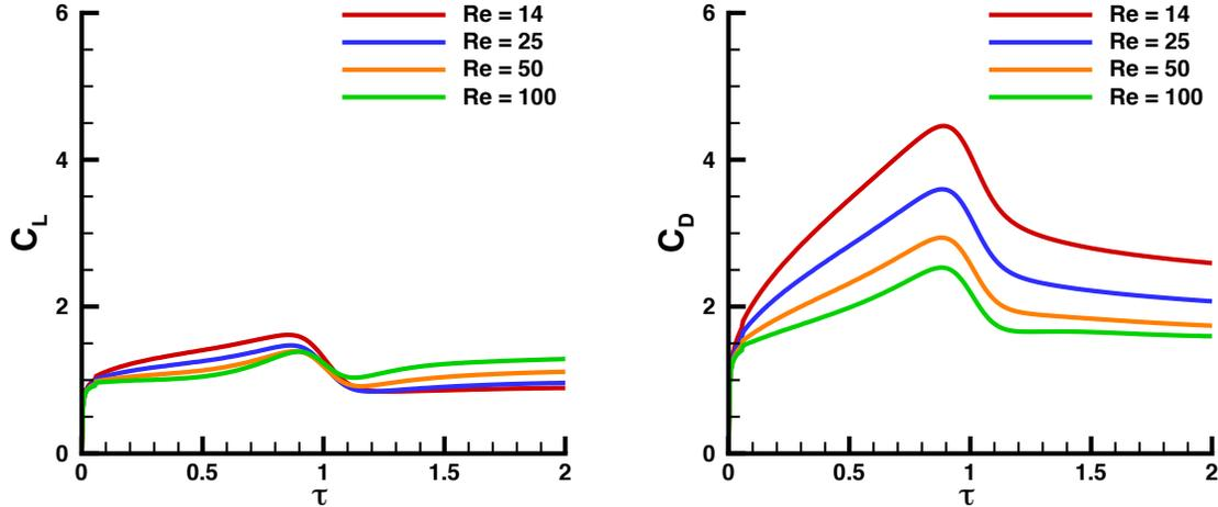
Figure 8. Reynolds number effect on the aerodynamic loading for  $AR = 4$  wing accelerating over one chord length of travel.
