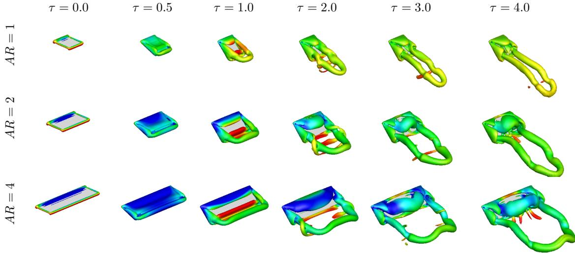
**Figure 5.** Flowfield images illustrating the effect of aspect ratio for a wing pitching over one chord length of travel at  $Re = 300$ . The vortical structure is visualized by an isosurface of  $Q = 3$ , colored in contours of constant pressure.
