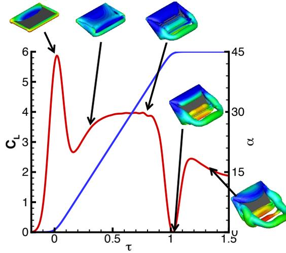
Figure 1. Coefficient of lift (red) and angle of attack history (blue) for an  $AR = 2$  flat plate pitching over one chord length of travel at  $Re = 300$ . The three-dimensional vortical structure is visualized using a  $Q$ -value of  $Q = 3$  and the isosurface is colored by contours of constant pressure.
