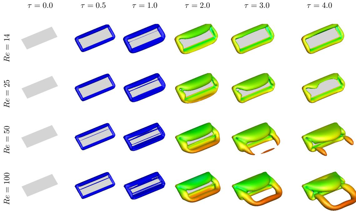
Figure 9. Flowfield images illustrating the Reynolds number effect for the  $AR = 4$  wing accelerating over one chord length of travel. The  $Q$ -value used to visualize all Reynolds numbers considered is given by  $Q = 0.5$ , and is colored by contours of constant pressure.
