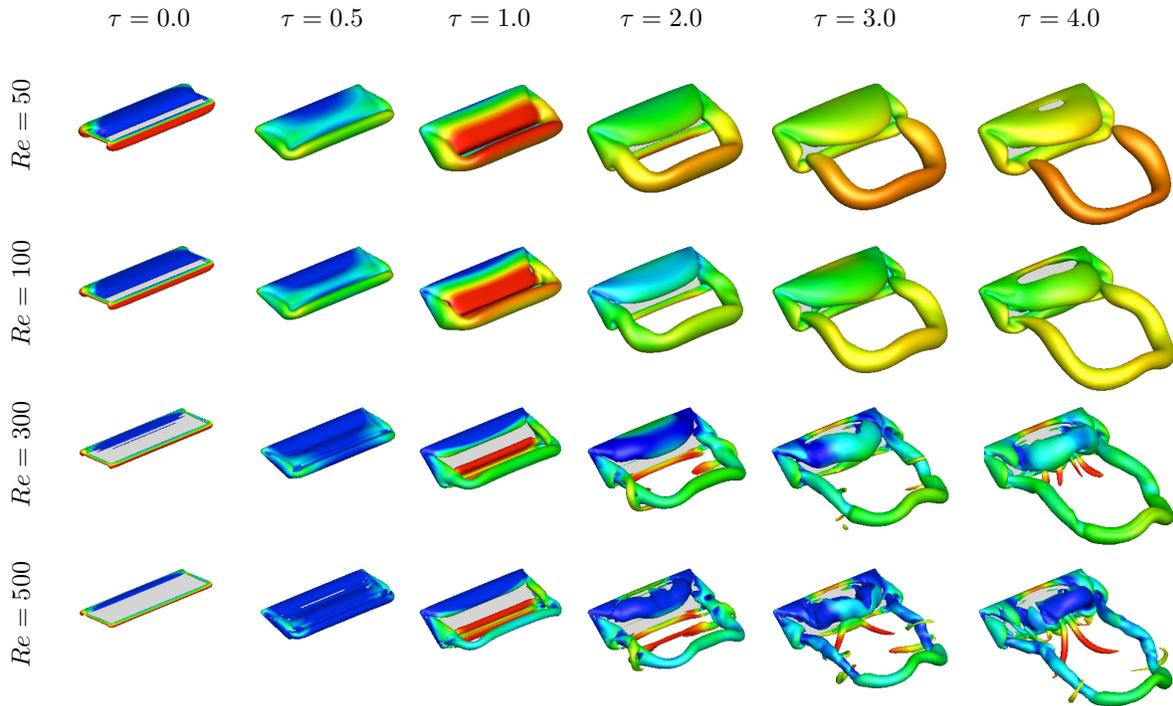
Figure 3. Flowfield images illustrating the Reynolds number effect for the  $AR = 4$  wing pitching over one chord length of travel. The  $Q$ -value used to visualize the vortical structure is given by  $Q = 0.5, 1, 3,$  and  $5$  for  $Re = 50, 100, 300,$  and  $500$ , respectively, and is colored in contours of constant pressure.
