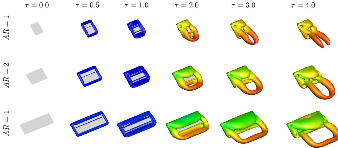
**Figure 11.** Flowfield images illustrating the effect of aspect ratio for a wing accelerating over one chord length of travel at  $Re = 100$ . The  $Q$ -value used to visualize all aspect ratios considered is given by  $Q = 0.5$ , and is colored by contours of constant pressure.
