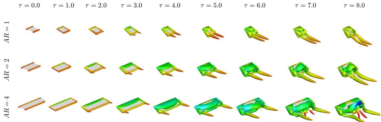
Figure 7. Flowfield images illustrating the effect of aspect ratio for a wing pitching over six chord lengths of travel at  $Re = 300$ . The wake vortices are visualized by an isosurface of  $Q = 3$ , colored by contours of constant pressure.
