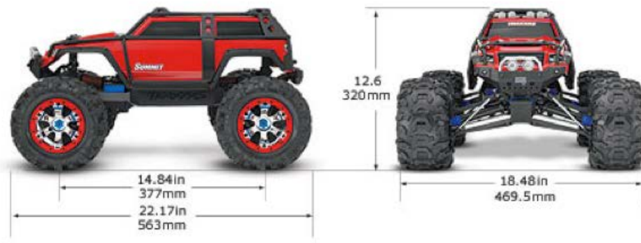
Figure 5. Dimensions of the Traxxas-Summit, from [7].
