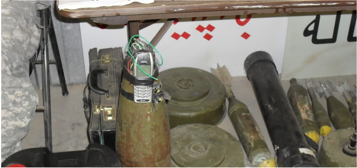
Figure 1. Cell-Phone Triggered Improvised Explosive Device
