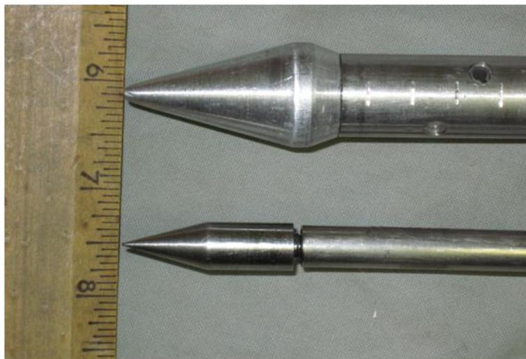
Figure 5-5. Cone and tip geometry for the Rammsonde (top) and Russian Snow Penetrometer (bottom). The scale on the left is in increments of inches.
