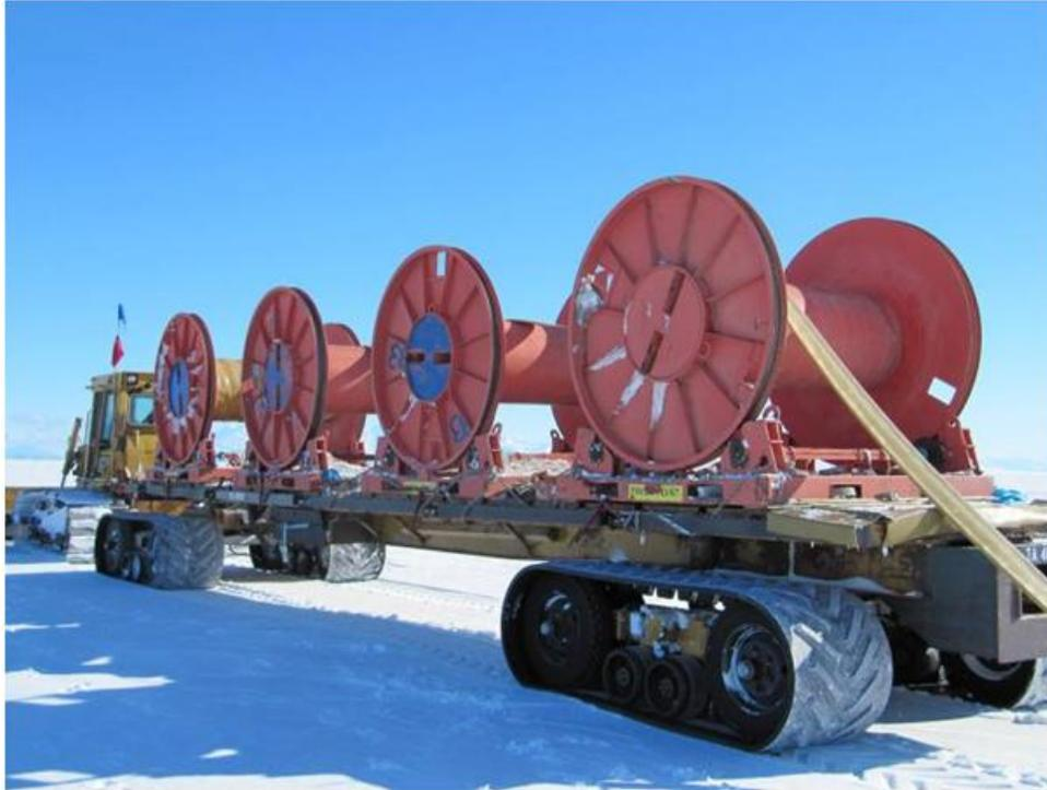
Figure 4-1. Use of challenger trailers to deploy flexible pipeline between Scott Base and PEG (photo courtesy of Alex Morris, RPSC).
