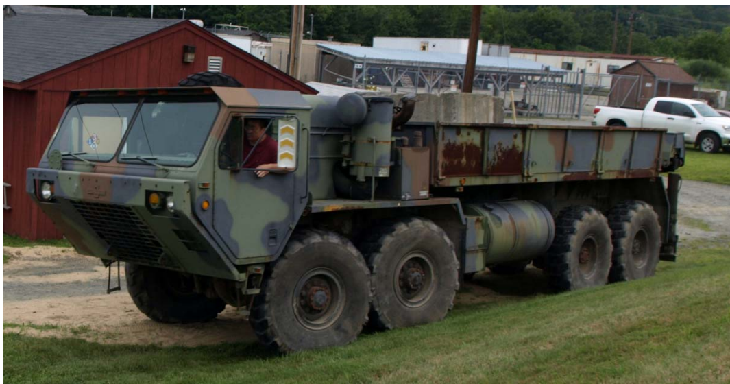
Figure 3. Heavy Expandable Mobility Tactical Truck (HEMTT). This 8 x 8 vehicle is steered with the two front axles with a total vehicle weight of 23,000 kg including payload.
