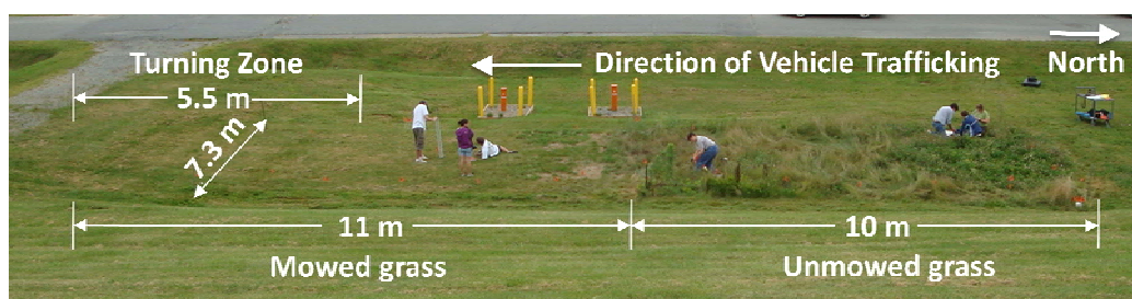
Figure 1. Outdoor test section. Test vehicle travels straight from North (right) to South across two treatments, mowed and unmowed grass, then turns in the last 5.5 m of the test section.
