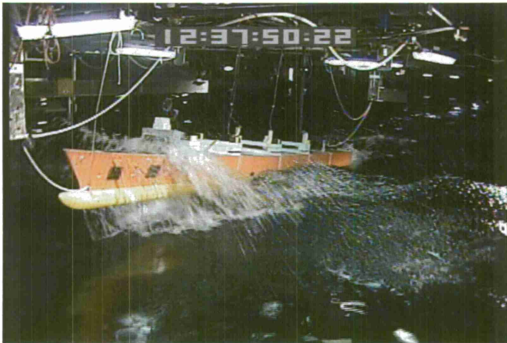
Figure 6. Run 478 deck house impact and extreme hogging moment.
