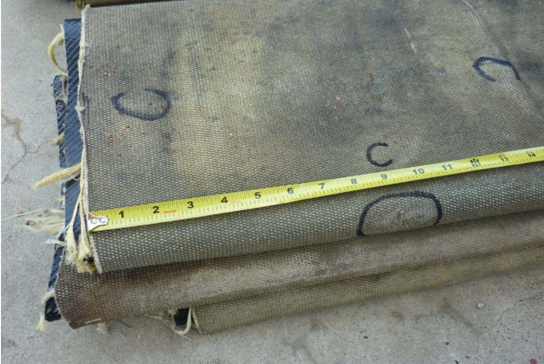
Figure 8. Abrasion to Outer Layer of Jacket of Specimen C
