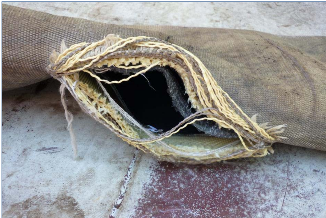
Figure 32. Specimen G Burst Testing Failure Close-Up
