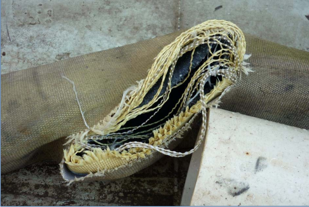
Figure 29. Specimen F Burst Testing Failure Close-Up
