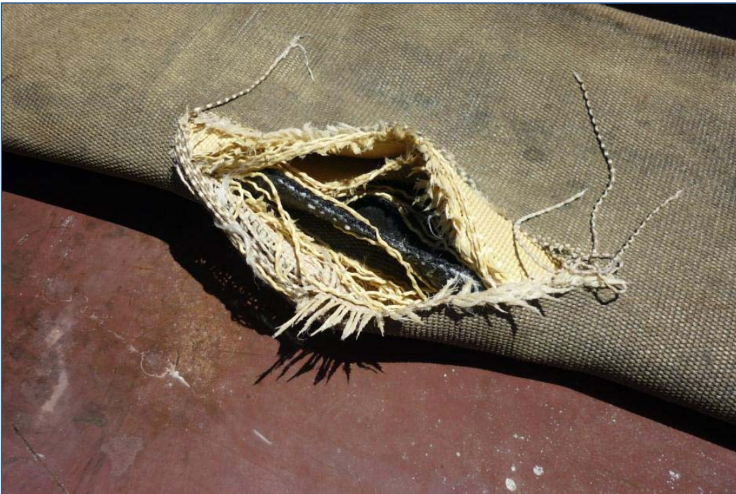
Figure 26. Specimen E Burst Testing Failure Close-Up
