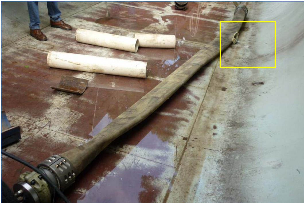
Figure 34. Specimen H Burst Testing Failure
