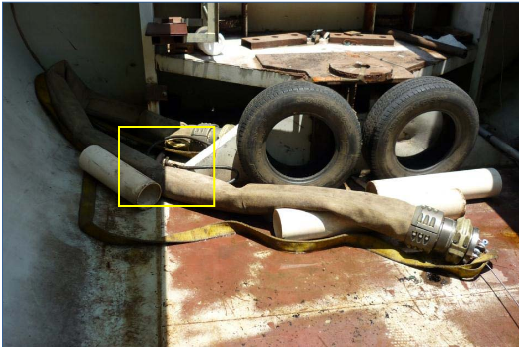
Figure 14. Specimen A Burst Testing Failure
