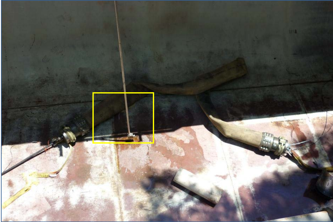
Figure 31. Specimen G Burst Testing Failure
