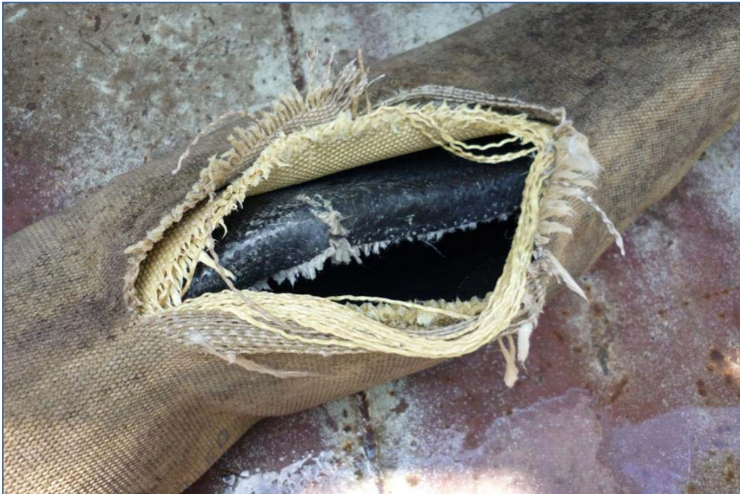
Figure 20. Specimen C Burst Testing Failure Close-Up
