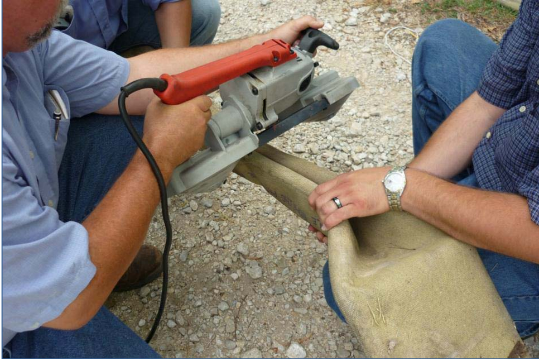
Figure 3. Cutting a Specimen with Portable Band Saw
