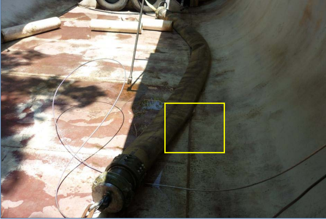
Figure 25. Specimen E Burst Testing Failure
