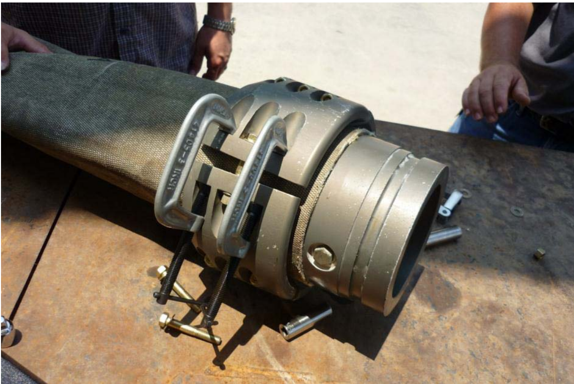
Figure 11. Installing End Fitting Collars
