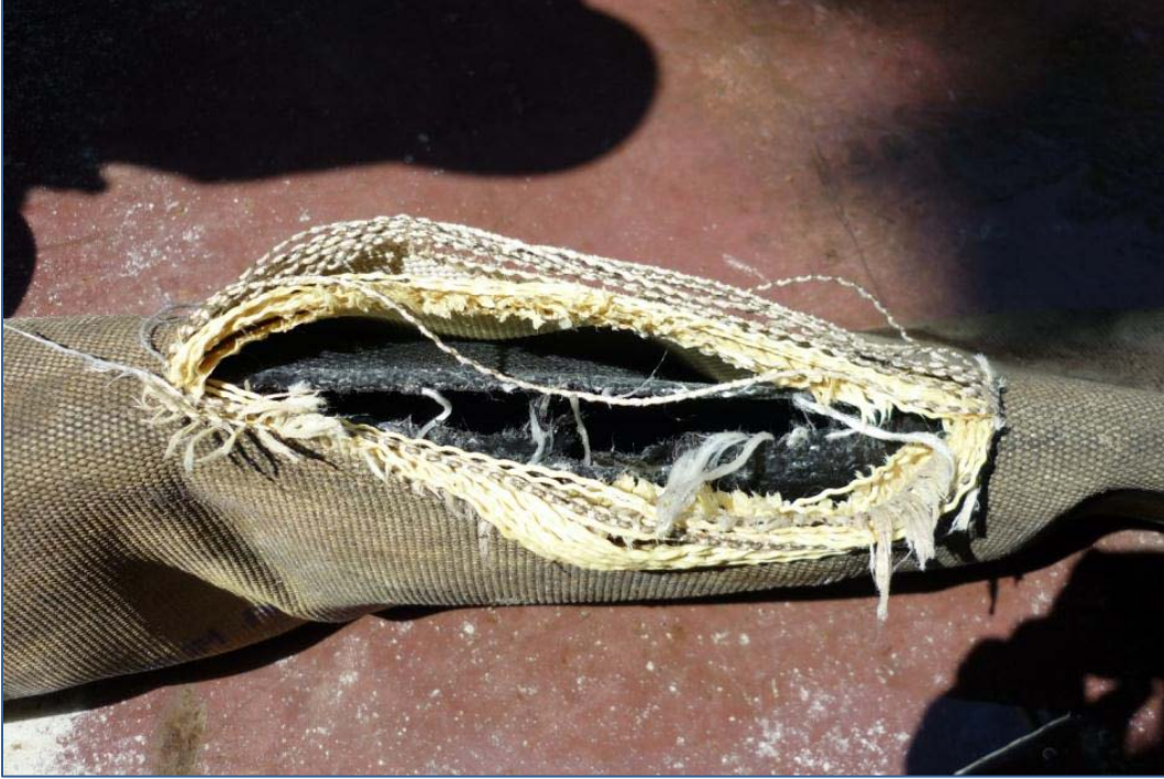
Figure 23. Specimen D Burst Testing Failure Close-Up
