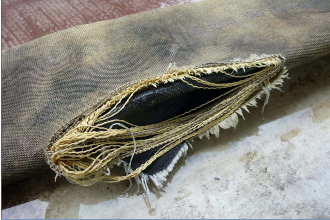
Figure 35. Specimen H Burst Testing Failure Close-Up
