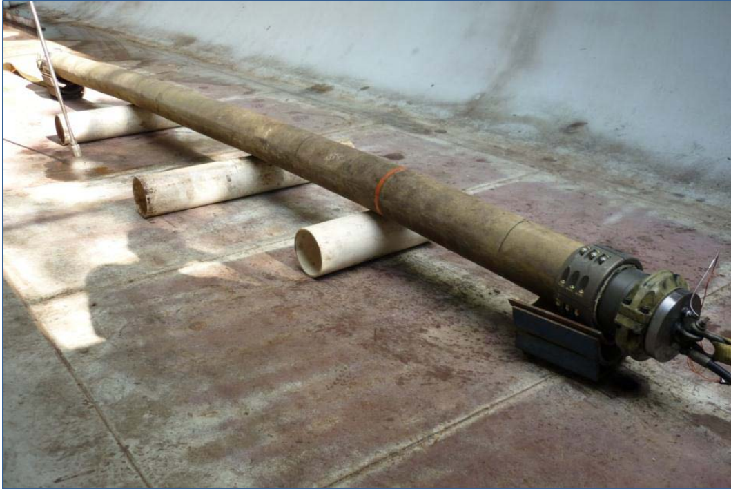
Figure 27. Specimen F Burst Testing Setup
