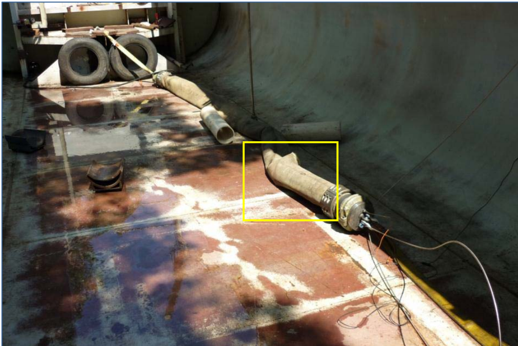
Figure 22. Specimen D Burst Testing Failure
