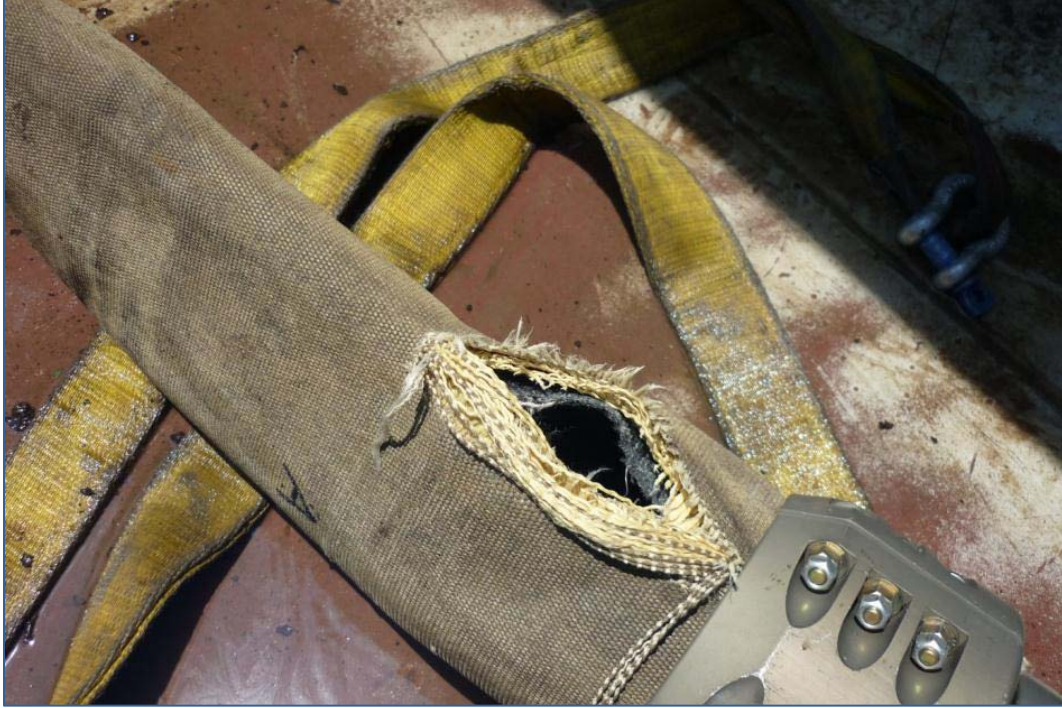
Figure 15. Specimen A Burst Testing Failure Close-Up
