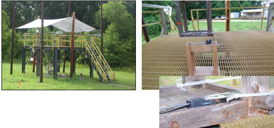
Figure 20. Photographs showing the test stand and a GMR sensor mounted on the test stand shuttle.
