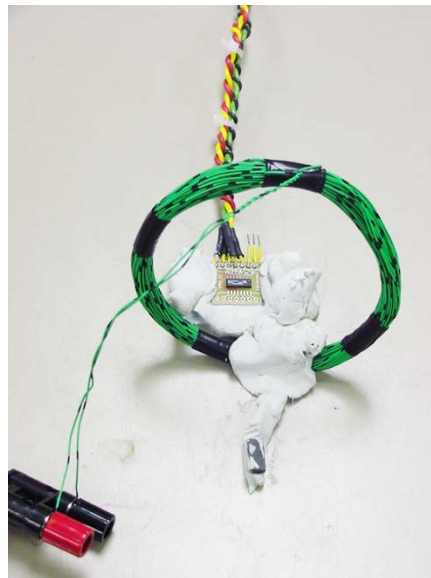
Figure 16. Configuration for non-linear biasing of a GMR sensor. A small magnet biases the GMR sensor part way up the linear portion of its operating curve (see Fig. 3). The coil adds further CW (AC) biasing so that any small perturbation of the biasing conditions causes a large change in GMR sensor output voltage.
