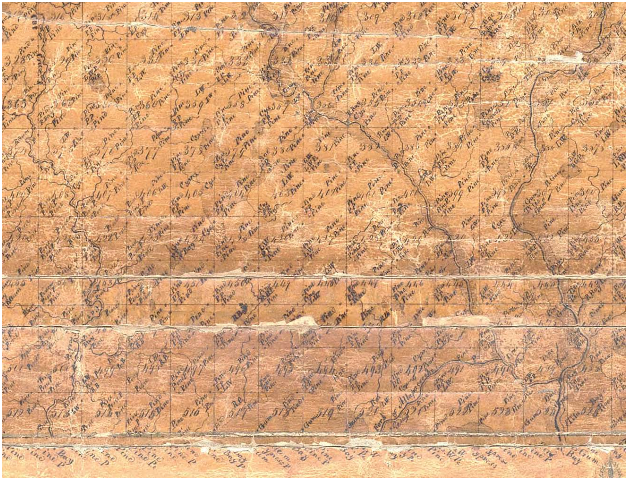
Figure 3. A portion of District 10 1820 Land Lot survey map. The north/south drain on the left is Cat Creek. From the upper center, Big Creek drains southeast into the Alapaha River. At lower right, Mill Creek is called “Fork of Allapacooche” (Allapacooche was Big Creek). Lots are numbered in their centers. At lower right, lots 522 and 523 include the northern half of Milltown Bay which is shown as a slightly darker shade than the rest of the map. At bottom center, lots 517, 518 and 519, also shaded, include the northern curve of Old Field Bay and its wet drains to the north. At the juncture of lots 446 and 447 (lower right center), Berryhill Pond can be made out, along with its drain Alligator Creek which can be traced south into Old Field Bay. Wetlands and stream drainages are much more reliable on this map than on that for District 11 below.
