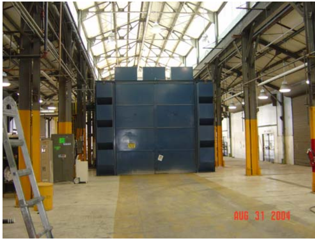
Figure 1. Shot blast booth in the Paint Shop.
