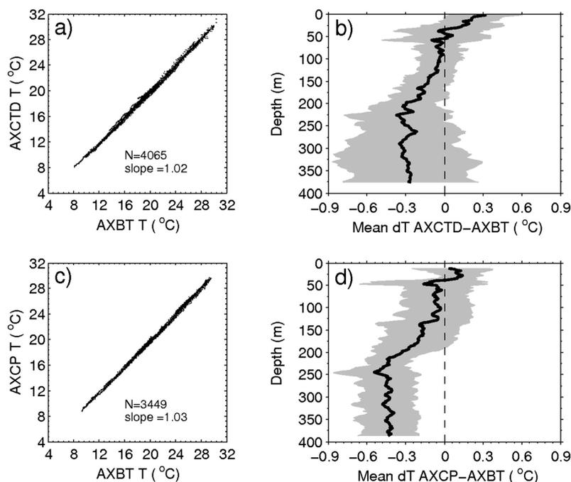
**Figure 2.** Comparison of temperature (°C) profiles from all WP-3D flights. (a, b) Air-dropped (or aircraft-deployed or airborne expendable bathythermographs (AXBTs) versus AXCTDs (22 sets). (c, d) AXBTs versus AXCPs (20 sets). (b, d) dT represents temperature difference, and the bold line and gray shadow represents the mean and standard deviation of this temperature difference, respectively.
