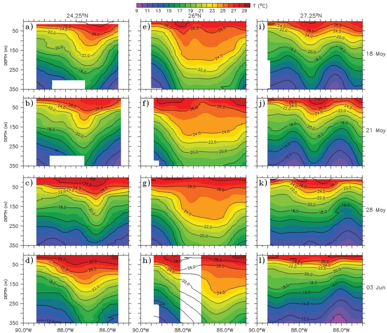
**Figure 4.** Objectively analyzed vertical sections of temperature ( $^{\circ}\text{C}$ ) from airborne profilers at (a–d) 24.25°N, (e–h) 26°N, and (i–l) 27.25°N. Blanked regions are points where the mapping error is larger than 60%.
