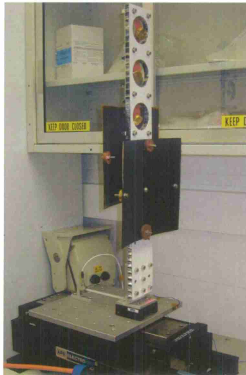
Figure VI-25: sub-assembly of a composite beam with hybrid bistable snap-through units.
