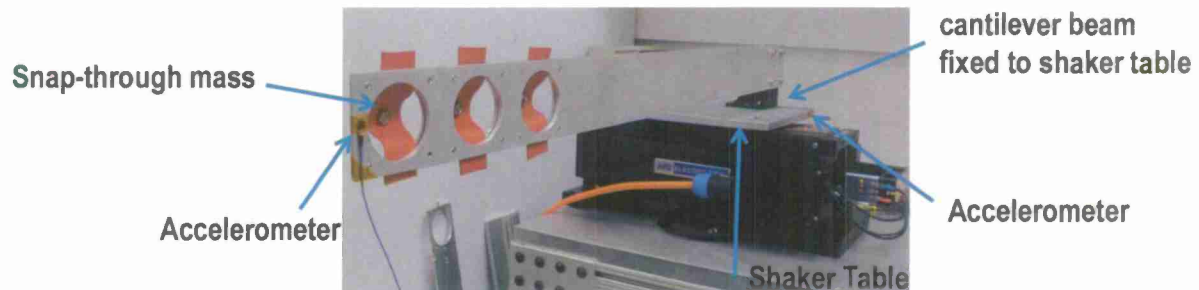
Figure VI-14: Experimental setup of the cantilever beam with attached bistable snap through units
