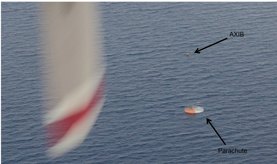
Figure 4. Deployment of the Airborne eXpendable Ice Beacon (AXIB) buoy 100181 from an Arctic Domain Awareness flight in August, 2012 (top). The picture below shows the AXIB deployed in open water at 78N 150W, and the parachute which separates from the buoy during deployment. The AXIB was developed by the USIABP specifically to survive annual freeze/thaw cycles in the harsher, dynamic conditions of the seasonal ice zone. Our ability to air drop AXIB makes it possible to fill holes in the IABP AON where we may not have deployment opportunities from ice breakers.
