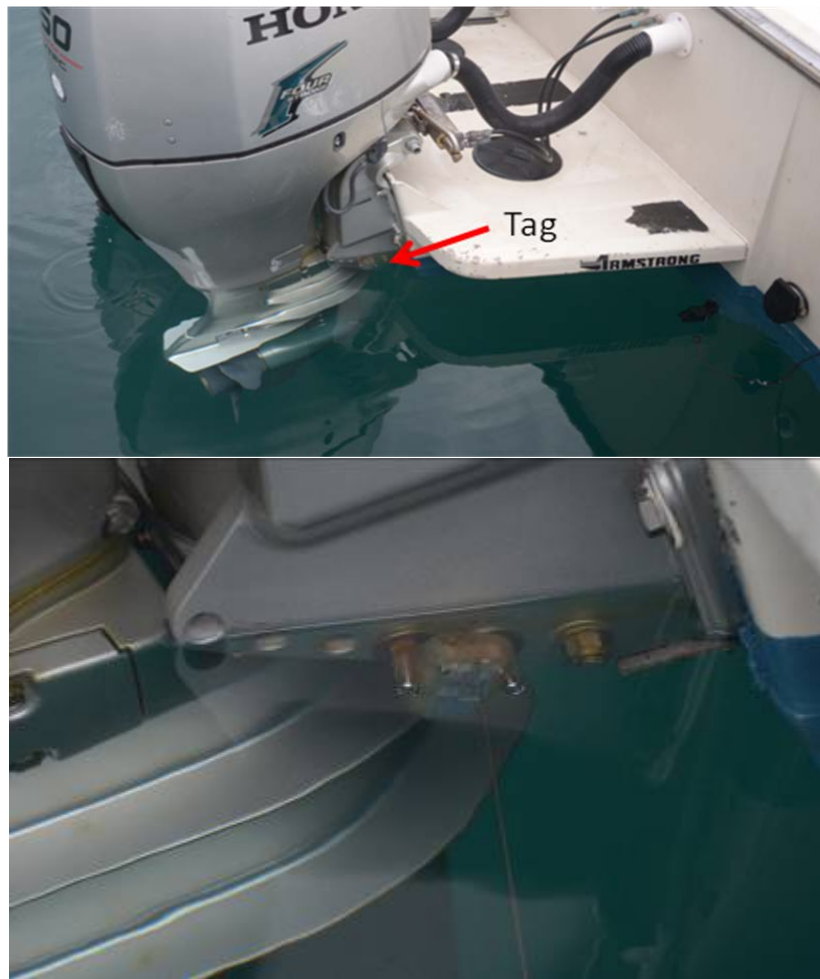
Fig. 14. Photographs of the new location-only SPOT100 AM-240C tag mounted to an outboard engine to examine resistance to strong water force and vibrations.
