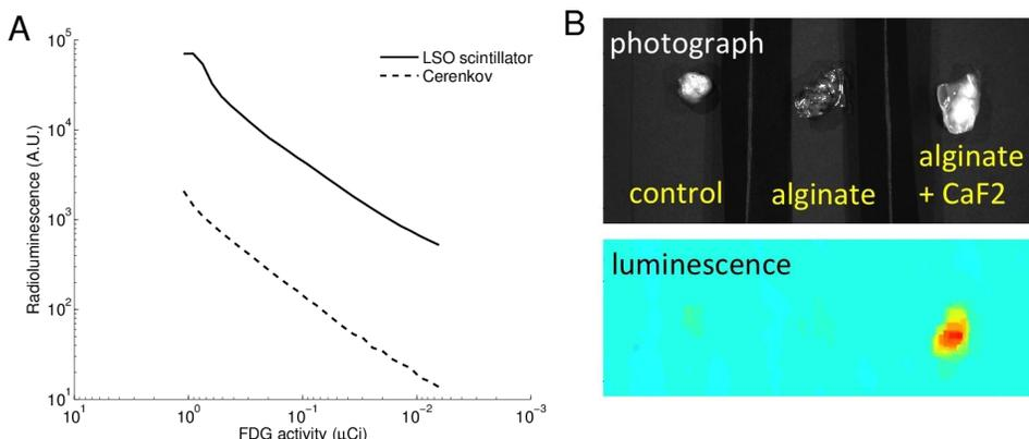
**Figure 3.** (A) Luminescence intensity shown for Cerenkov luminescence and LSO scintillator. The scintillator provides  $\sim 30\text{X}$  signal enhancement. (B) Luminescence enhancement shown for a flexible scintillator film, applied directly on an excised tumor specimen.
