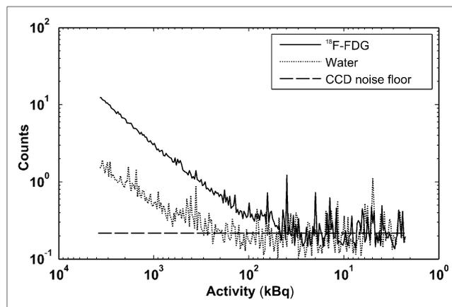
**FIGURE 2.** System sensitivity via sequential imaging of 3.7 MBq (100  $\mu$ Ci) of  $^{18}\text{F}$ -FDG for approximately 20 h. Optical signals from  $^{18}\text{F}$ -FDG and control sample were plotted.
