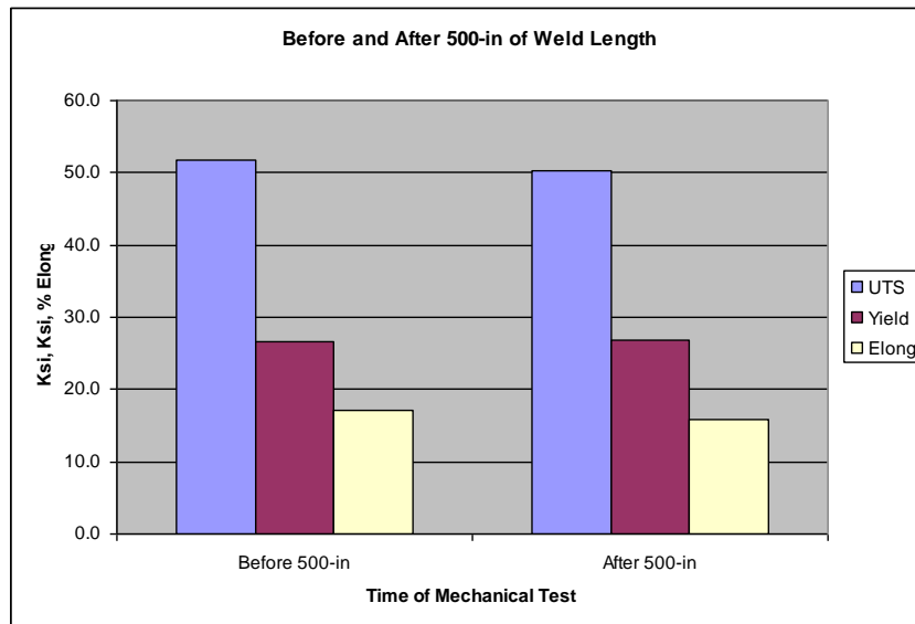
Figure 4. Static Tensile Properties from the Tool Life Test using Tool No. 51316-T06
