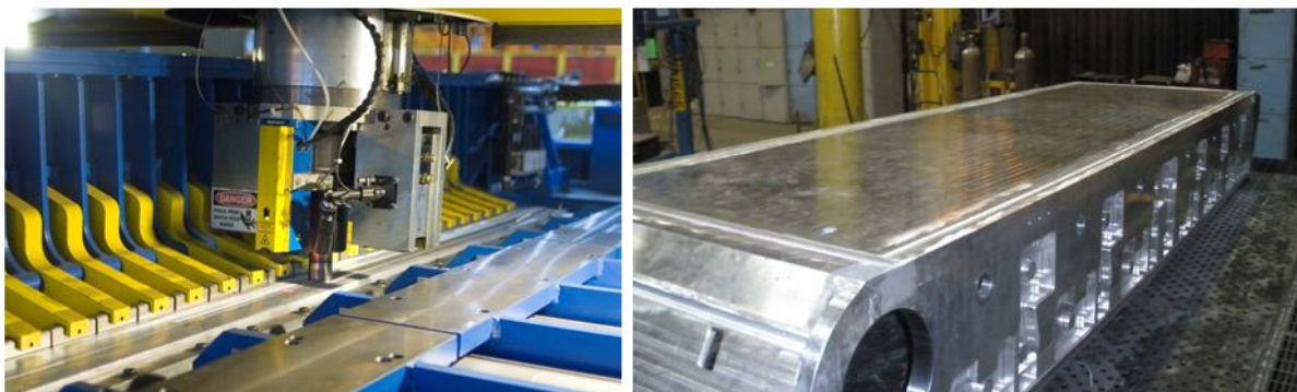
Figure 10. Military Vehicle Demonstrator during Welding (Left) and Fully Assembled
