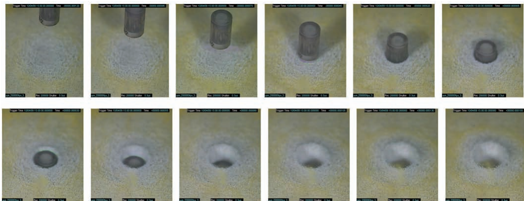
Fig. 6 High-speed visualization of detailed behavior of projectile during penetration. (Frame rate; 200,000 fps (every 5 frames), exposure time; 300 ns, impact velocity; 495 m/s.)
