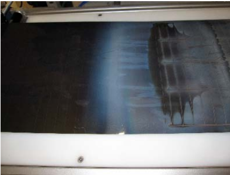
Figure 1.1.8 Picture showing damage to the ITO target.
