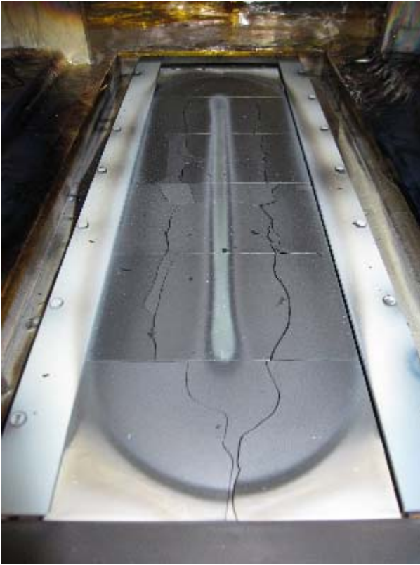
Figure 1.1.8 Picture showing damage to the ITO target.
