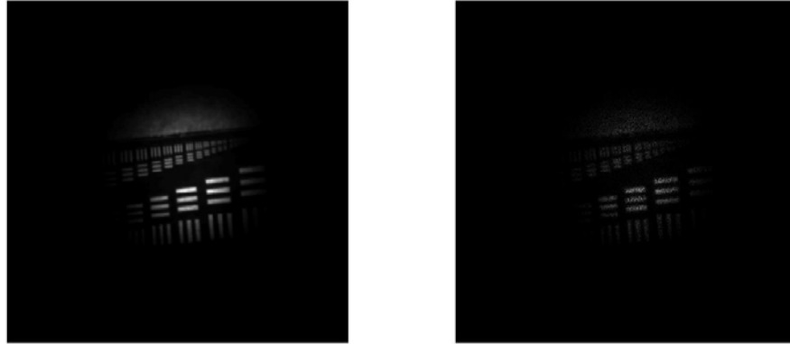
(a) (b) Fig. 1 Incoherent imaging and coherent imaging with only speckle noise
