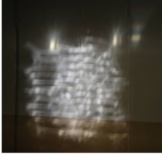
Figure 6. Solar panel reflection off a flat surface. This figure illustrates the complex 2-D pattern of individual tip-tilts from solar cells.
