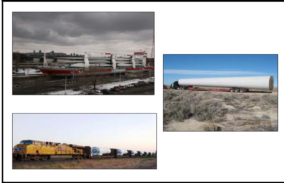
Figure 5. Modes of Wind Turbine Transportation
