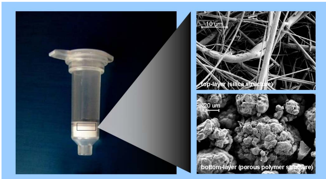
Figure 4: Scanning electron microscope photograph of spin column
