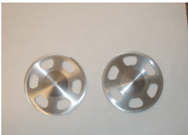
Fig. 3.13 Two versions of magnetically permeable “plasma” exit grids.
