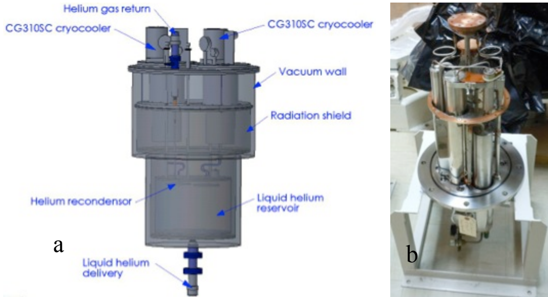
Fig. 3.19 a) Semi-transparent solid model for the helium recondensing cryostat, and b) digital image for one of the Daikin three-stage cryocoolers.
