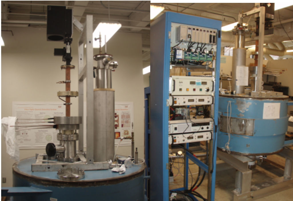
Fig. 3.14 Equipment assemblies. At left, ion source with RF assembly mounted on diagnostics flange atop the superconducting test magnet. At right, the rack-mounted ion source power supplies.
