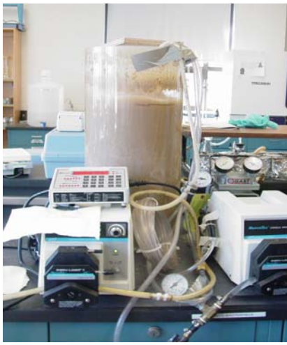
Figure 2.3: The lab-scale MBR in operation.
