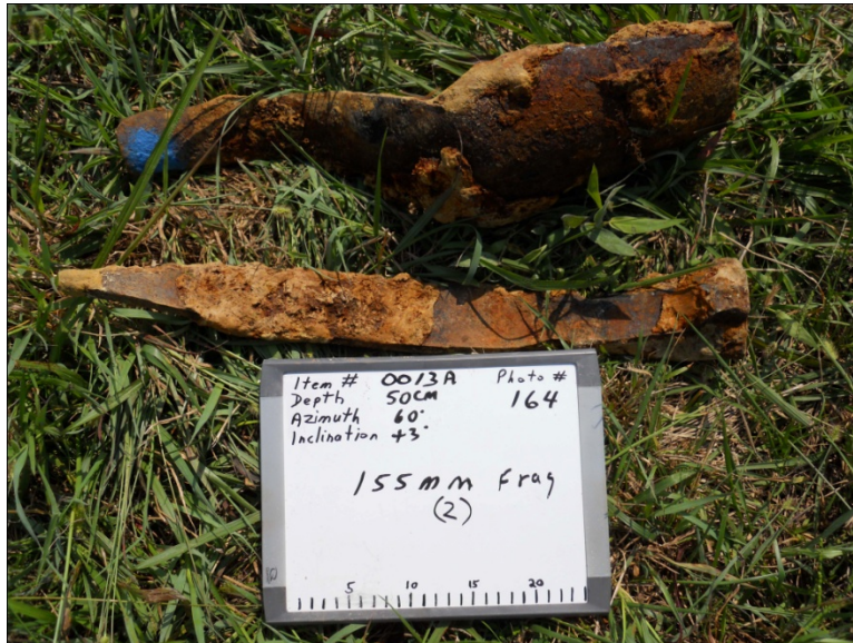
Figure 5-14. Photograph of the two objects responsible for anomaly 13 at Camp Butner.
