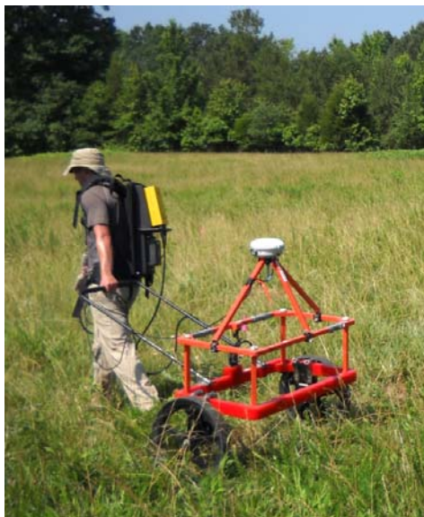
Figure 3-2. EM61-MK2 cart deployed at Camp Butner.
