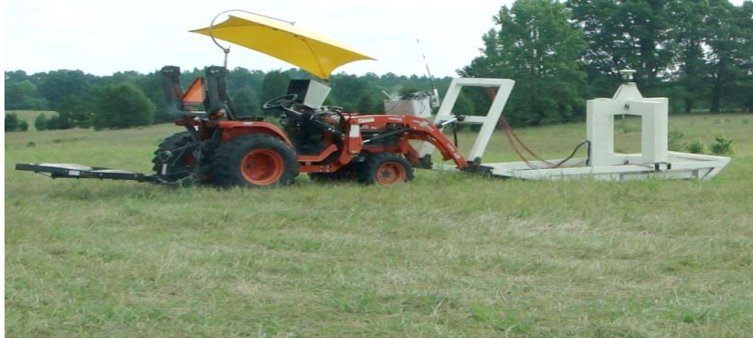
Figure 3-5. MetalMapper configured to collect survey data at Camp Butner.
