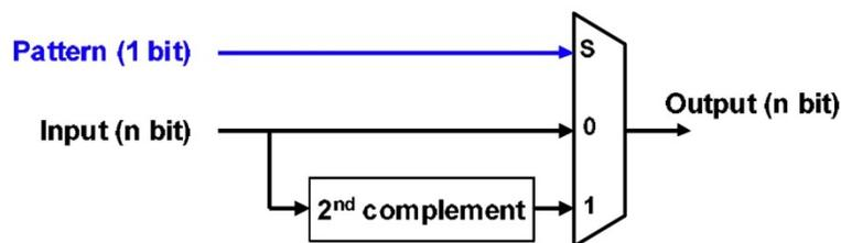
**Figure 2.14 Multiplier implementation for match filter.**
