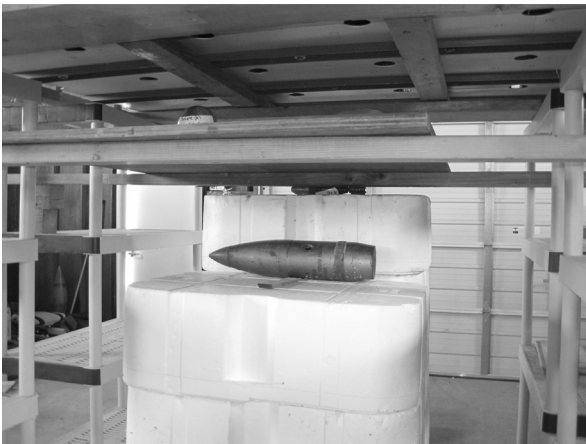
Figure 2. A test-stand experiment featuring an increasing number of targets under interrogation by TEMTADS. As in Figure 1, the system is observed essentially head-on from the +\hat{\mathbf{y}} -direction.
