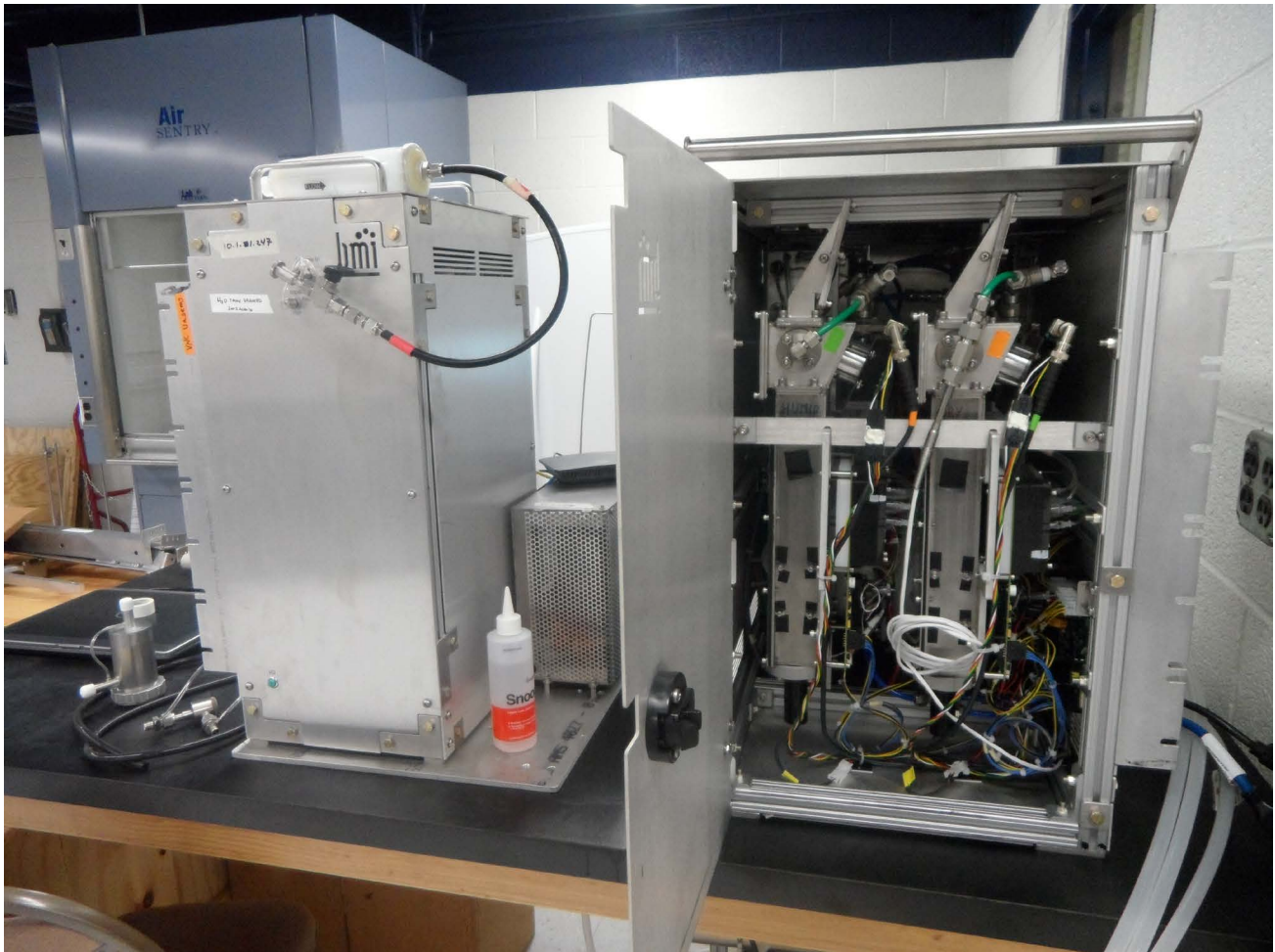
Figure 2. Photograph of the newly-developed differential aerosol sizing and hygroscopicity probe (DASH-SP). The left compartment is the differential mobility analyzer (DMA), which selects dried particles of a given size, which are then transported to the right compartment. The latter compartment splits the monodisperse stream into two streams: one is kept dry and the other humidified to a pre-selected relative humidity between 5-95%. These two streams then enter custom-made optical particle counters to quantify the final wet size. The final parameter of interest is the “growth factor”, which is the ratio of the humidified particle diameter to the dry diameter.
