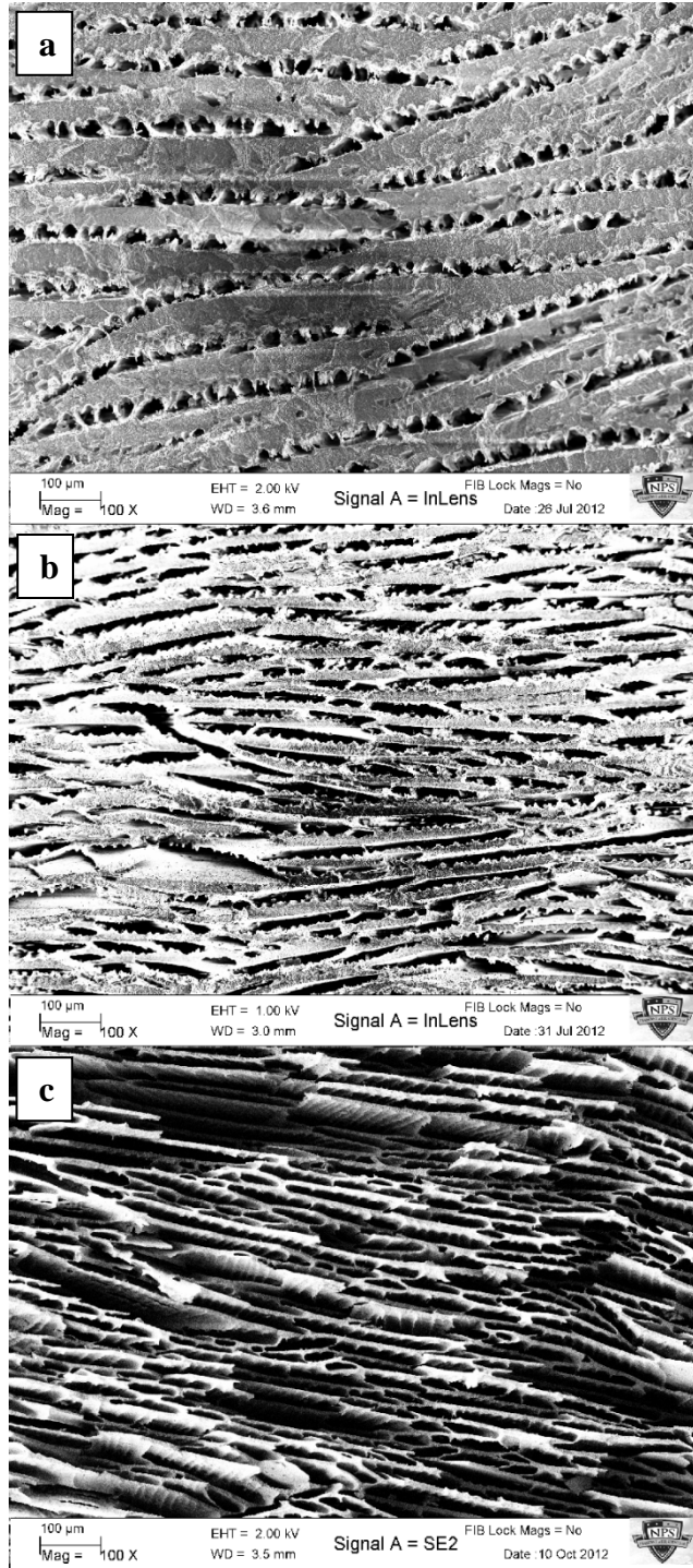
Figure 7. SEM micrograph showing the microstructure of samples with different porosity. The cross-section is parallel to the ice front. Total porosity of (a) 46 % (b) 60% (c) 75%.
