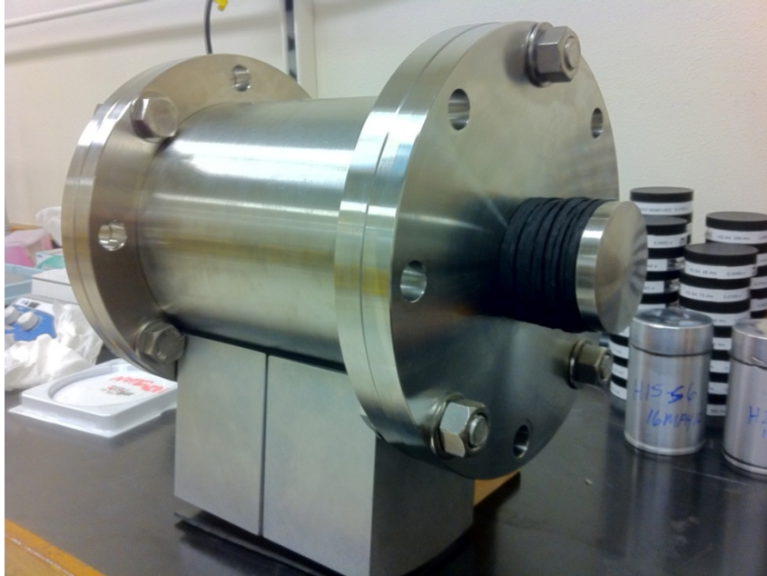
Figure 13. Fragmentation containment unit, assembled photo (From Ref. 5).
