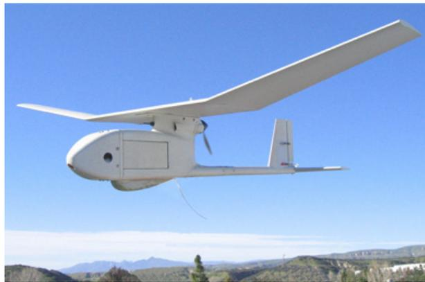
Figure 29. The AeroVironment Raven RQ-11 *UAV* (manufacturer's image).
