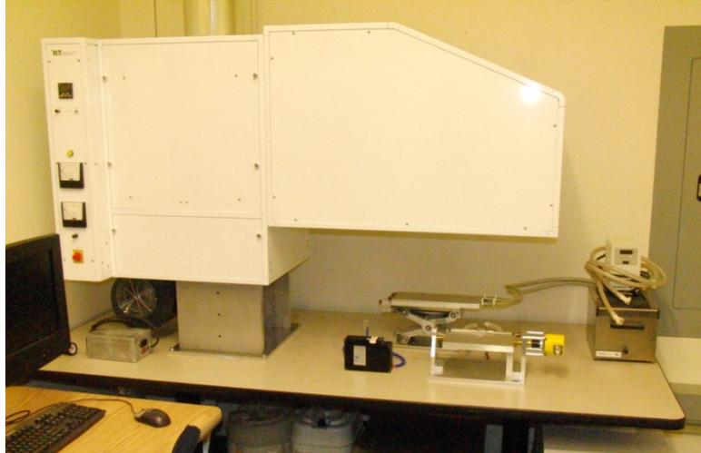
Figure 31. The RST Solar Simulator (From [25]).
