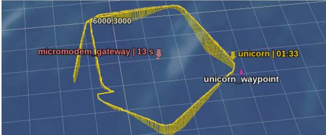
(b) A snapshot of the runtime visualization of the AUV “Unicorn” performing a sinusoidal depth excursion while performing a pentagon shape. While full, updates are delayed, the LAMSS\_STATUS\_FILLIN and LAMSS\_CTD messages give a detailed history of the vehicle’s track when the communication environment permits.
